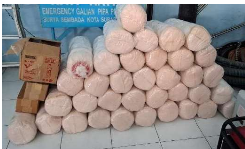
Gambar 3. Stok Anoda Magnesium di Gudang PDAM (15kg)
