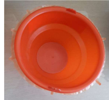
Gambar 7. Cacat plastic flash
